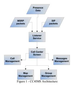
The core module of the CC4IMS is a Listener Service, which concentrates the SIP messages from the call-related IMS signaling, the MSRP messages for the chat related content and finally the Presence messages from the XDMS and Presence server of the IMS.
