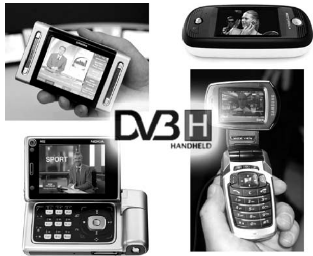
Fig. 5 Prototype DVB-H/cellular terminals
