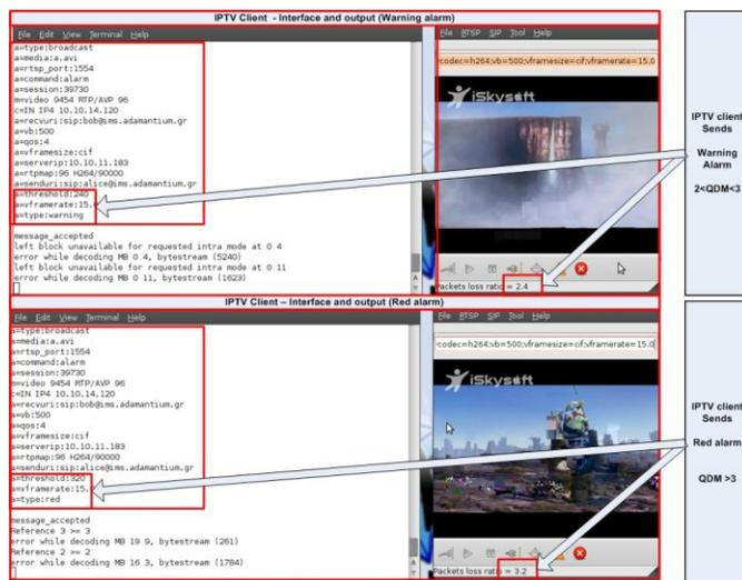
Figure 6. Warning or Red Alarm steps on IPTV Service
