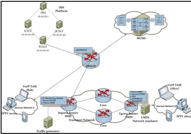
Figure 10. The small scale prototype topology
