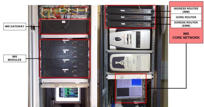
Figure 9. In-LAB testbed basic entities
