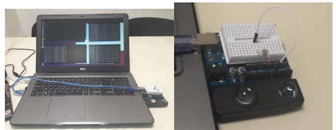
Fig. 3. Experimental CPE with VLC receiver and Arduino photodetector
