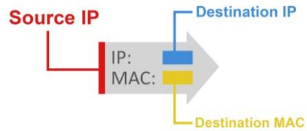
Fig. 4. Label used to show the SDN-based traffic steering commands per hop
