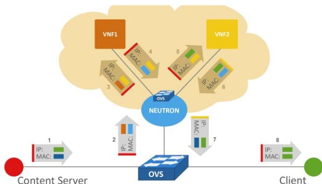
Fig. 3. Openflow-based traffic steering within Openstack platform
