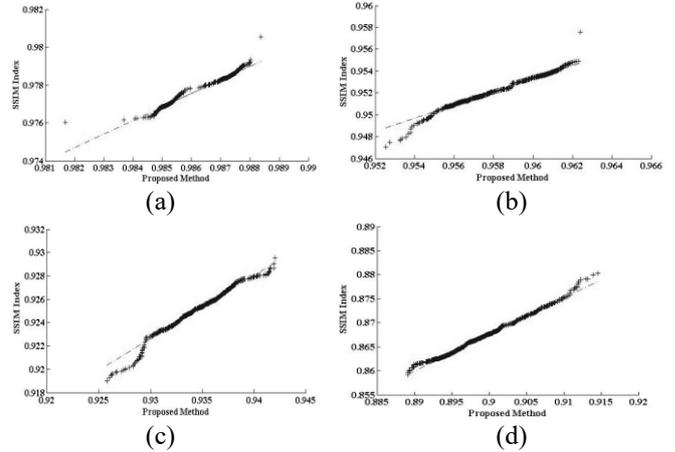
Fig. 6.  $Q-Q$  plots of the SSIM index vs. IS-QoE for the test signal Kristen&Sara at QP (a):12 (b):22 (c):32 (d):42
