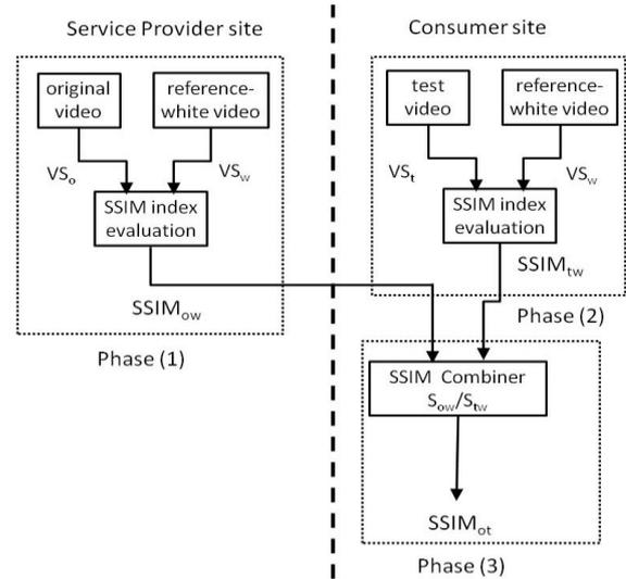
Fig. 1. The proposed approximated SSIM with relative point of reference
