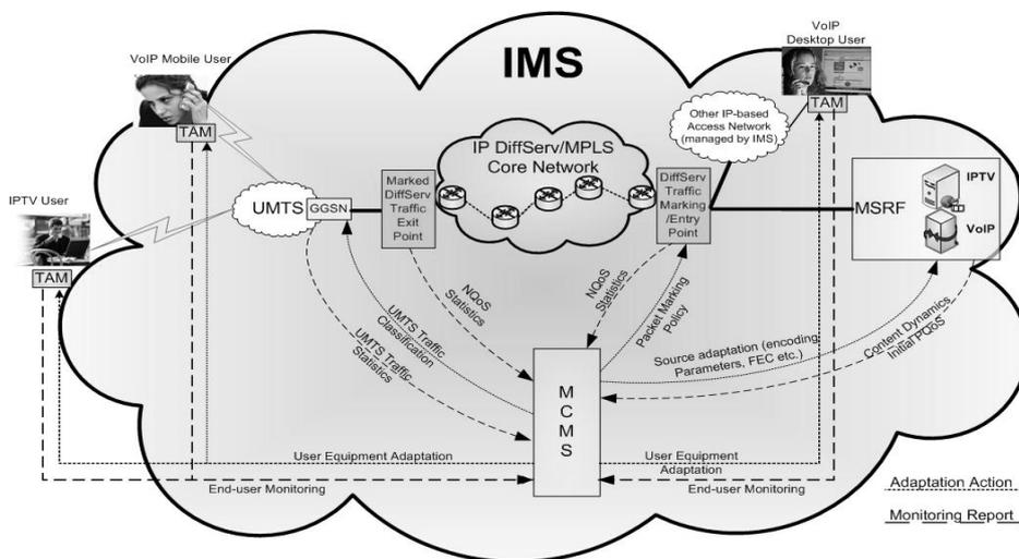
Figure 2: The overall architecture of ADAMANTIUM project.
