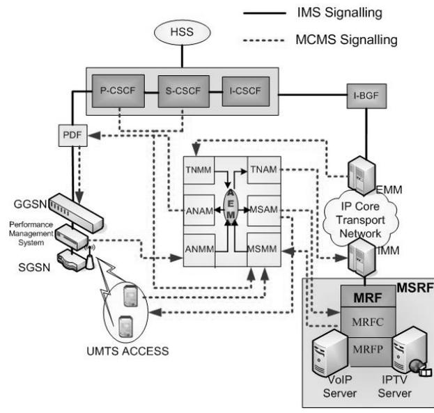
Figure 3: The ADAMANTIUM MCMS and NGN IMS architecture
