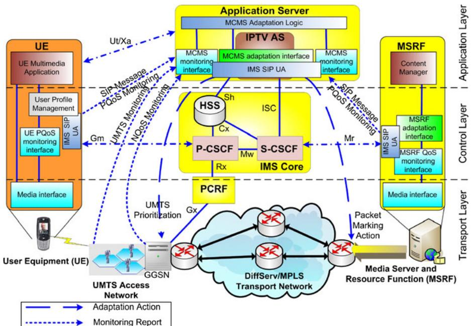
Fig. 2 New IMS-based architecture with PQoS mechanism
