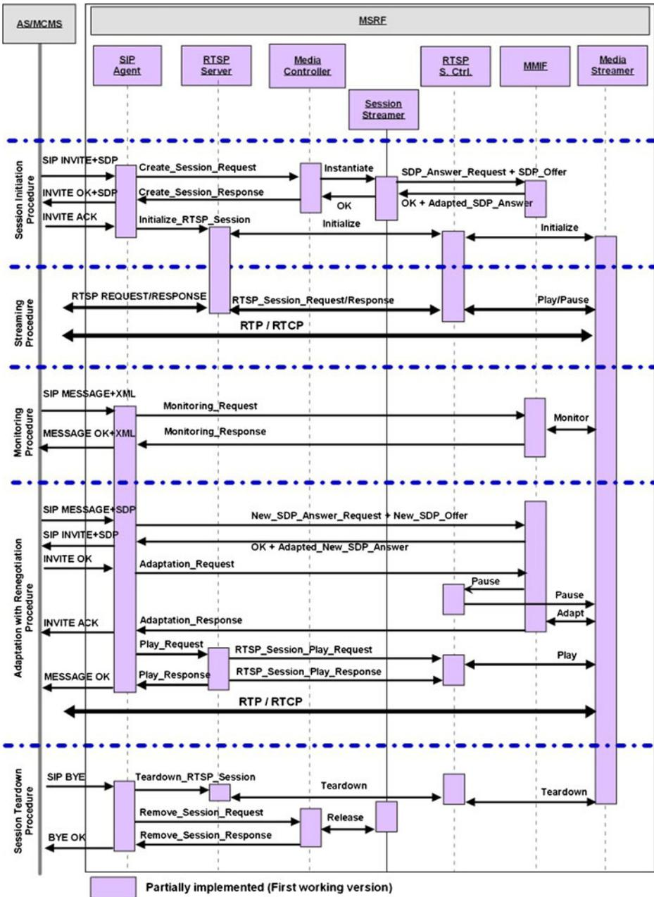
Fig. 8 MSRF adaptation procedure
